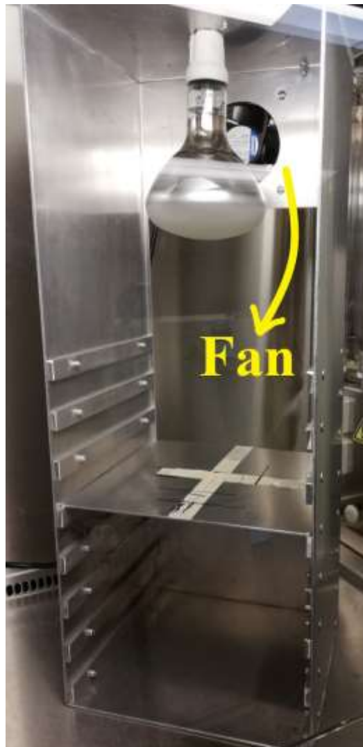
Figure G.1: Chamber used to assess the toxicity of TiO 2 based nanoparticles under simulated solar radiation.
