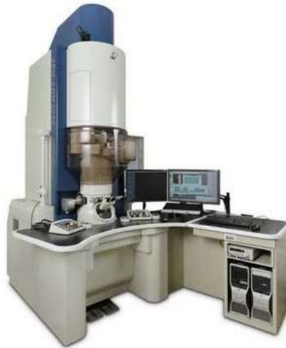
Figure 3.5: JEOL JEM-ARM200F Cs Corrected S/TEM [127].
