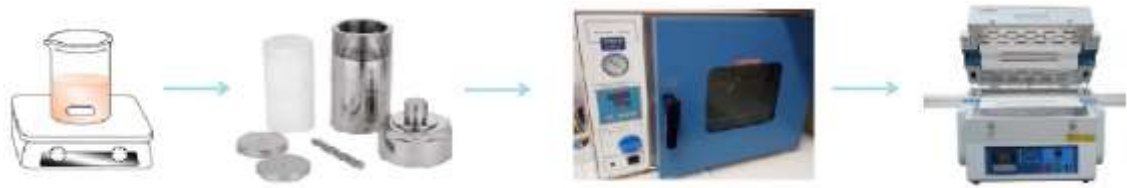
Figure 3.1: Schematic diagram of the procedure of the hydrothermal synthesis of \text{TiO}_2@Y_2O_3 nanoparticles.
